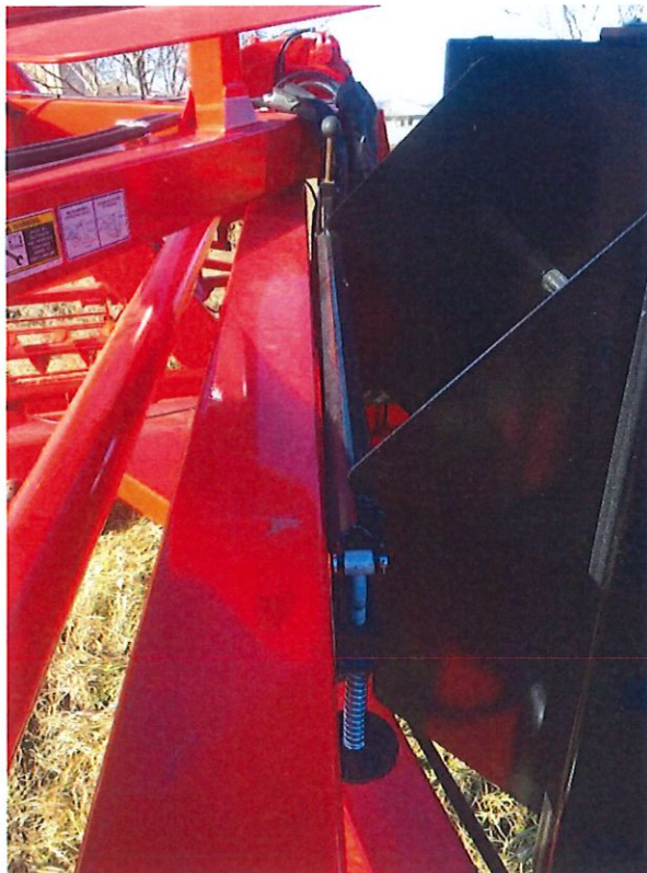
GBR300 Position against the Unloader Frame when not in use
