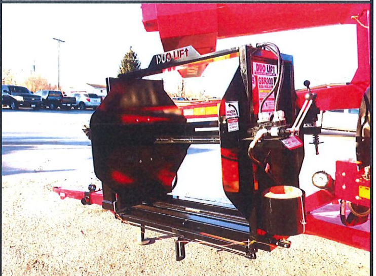
GBR300 Positioned and Locked in Transport Position
