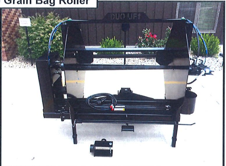
Bolt-On Tongue Jack Bracket, Machine Pivot Lock Handle, and Sliding Twine Wrapping Handle
