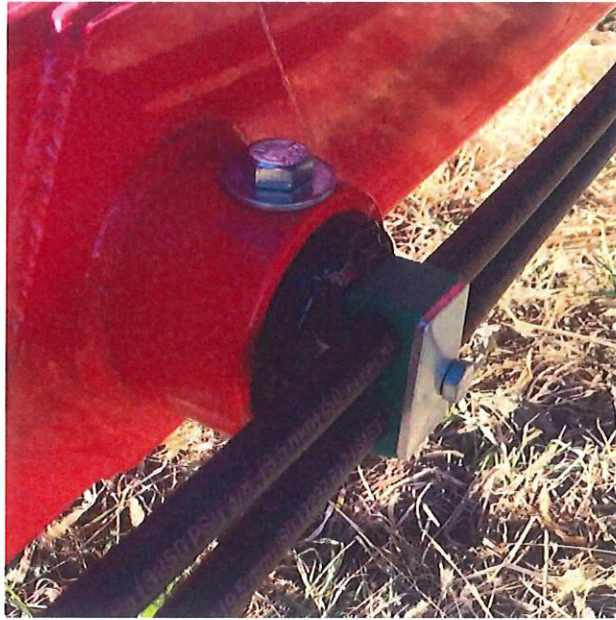
Route Hoses Rearward and secure with Hose Holder installed in original Tongue Jack Location
