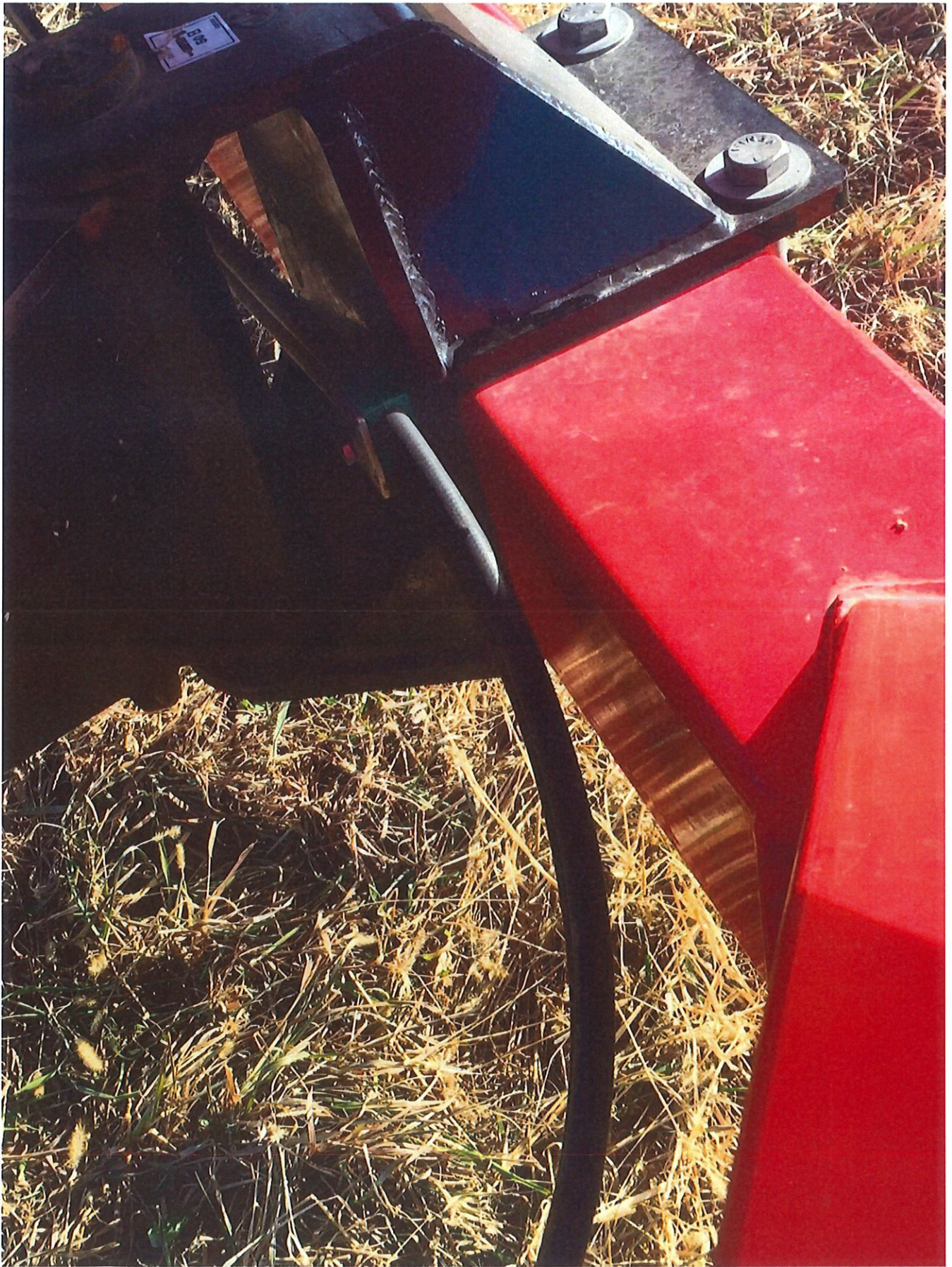
Hoses are secured and routed rearward with Hose Holder provided on GBR Mounting Bracket
