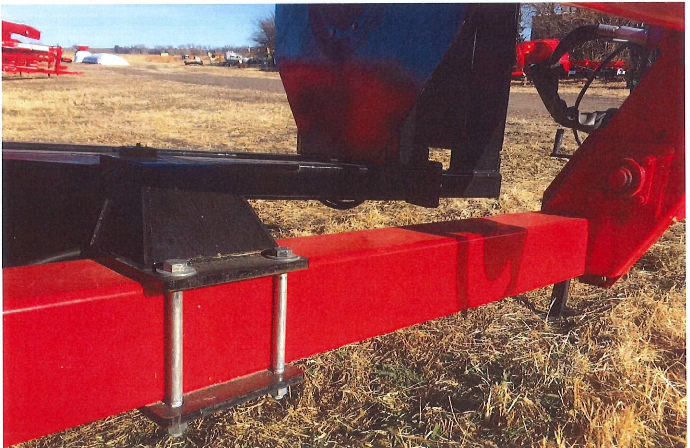
Position and Secure GBR Mounting Bracket 46" Rearward of PTO Support Structure
