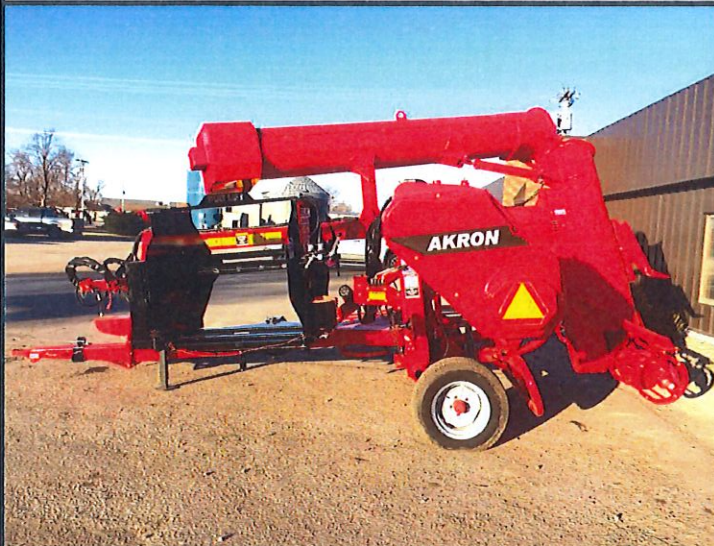
GBR300 Mounted to an Akron EXG300X Grain Bag Unloader
