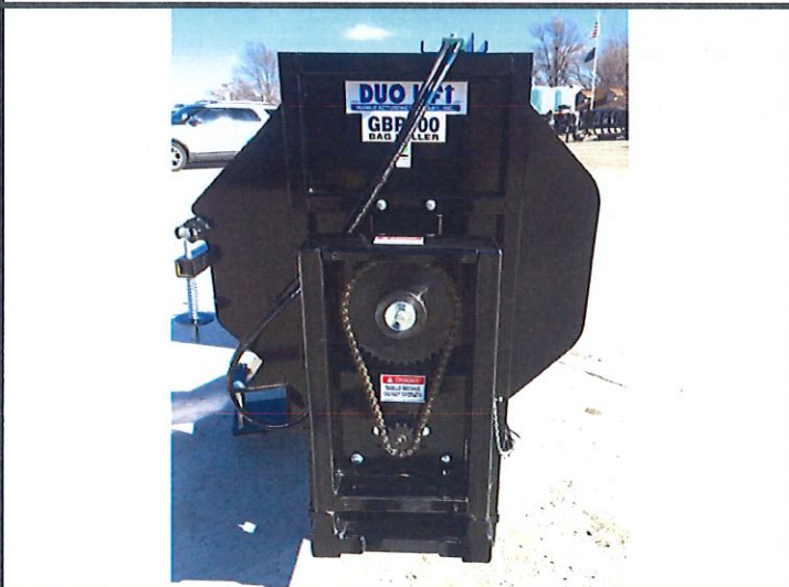
Spear and Rotor Drive System with Easy to Adjust #60 Drive Chain
