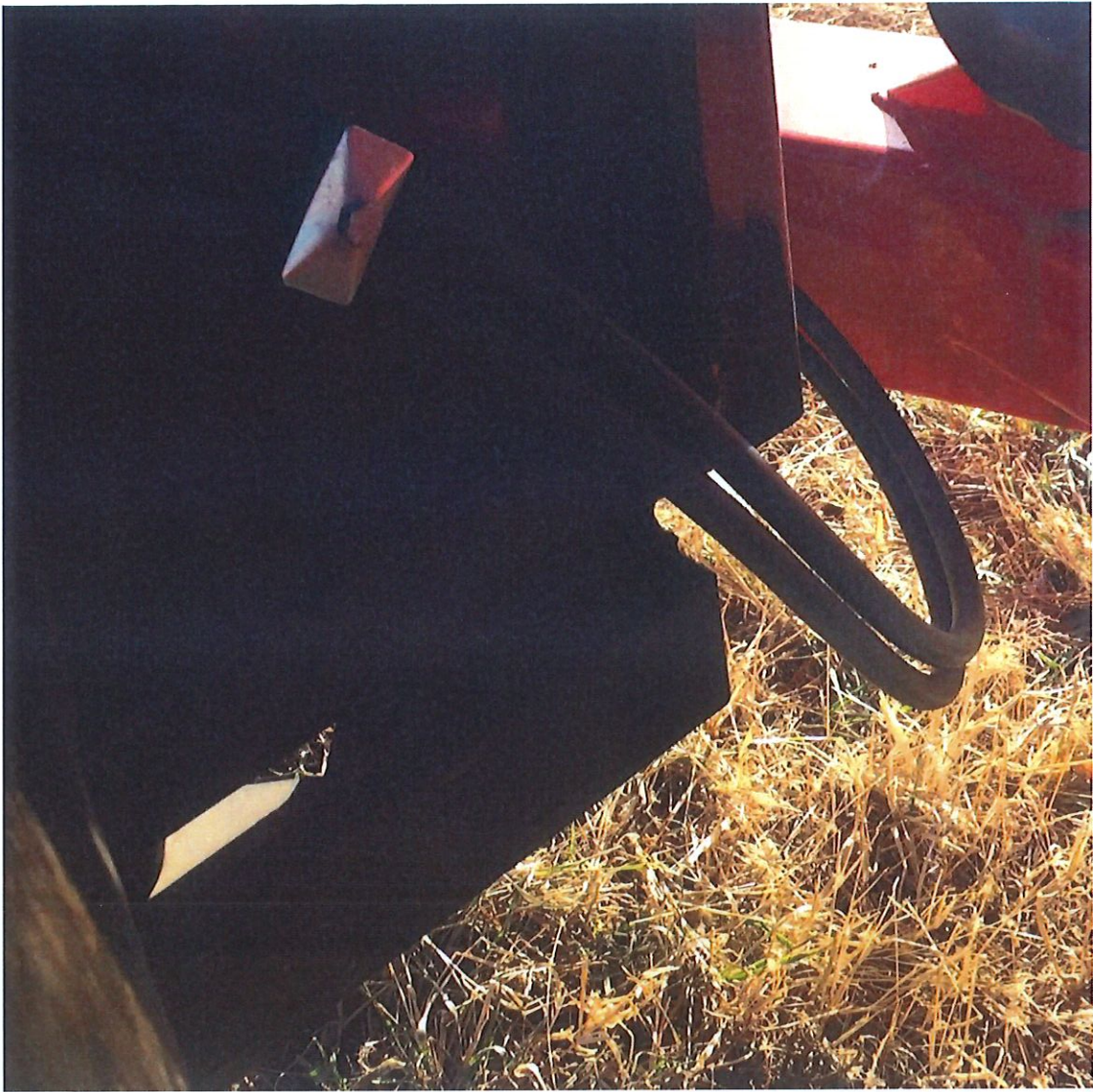
Secure Hoses through the Hose Holder on GBR300 Side Sheet
